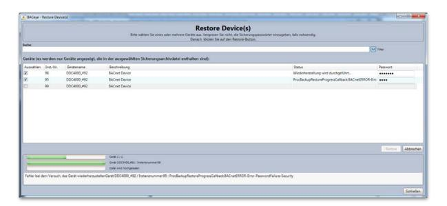
The status of the restoration of the respective device and its result is shown in the Status column. In addition, information about errors and about completion of the operation is shown in the text field below the progress display.
