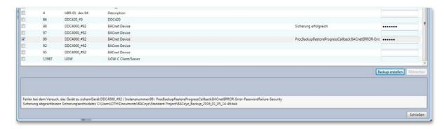
After the backup has been completed, the backup file contains all successfully completed backups. Unsuccessful backups can be repeated by pressing the <Create backup> button again. There is no new check of the destination file here. Instead, if a repetition is successful, the backups are added to the existing backup file. The same applies if other devices are marked after a backup has been created. However, existing backups are not replaced by renewed marking of the corresponding devices.
