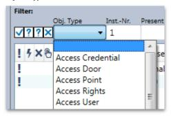
The object type can be filtered using a selection list. The list includes all possible object types. This also includes all types of proprietary objects if the device defines them.
