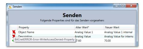
It is possible to also use the <*Log>* button to find out the reason why the send process was not successful. The transmission log can be called with the <*Log>* button to obtain further information on the problem which has occurred.
