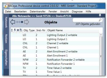
When "Device" is double-clicked, BACeye navigates to the "Object" hierarchy level. BACeye displays all objects found in the selected device in the object list.
