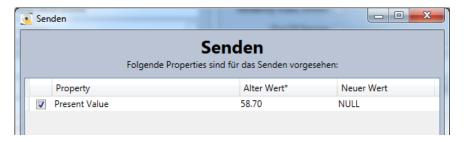
At this point and via the checkboxes to the right, it is possible for the user to deselect individual properties and not yet write them. If properties are deselected, the changes made are not lost; they remain available for a further write process.
